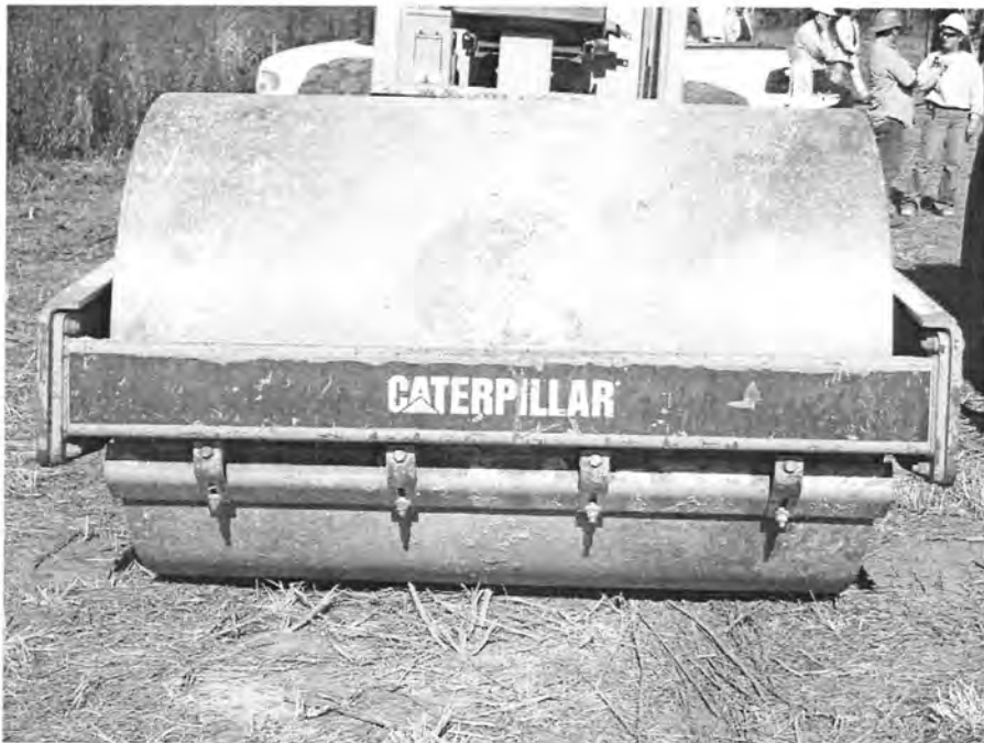
Figure 73. Steel Drum Roller Used for Final Compaction
