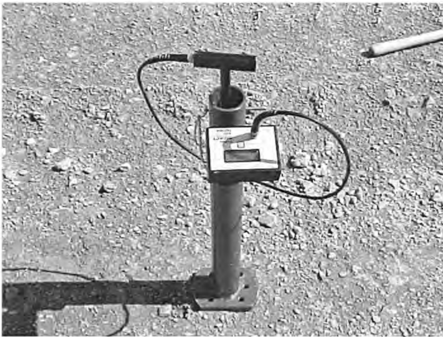
Figure 78. Clegg Impact Hammer
