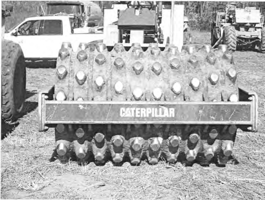
Figure 72. Vibratory Padfoot Roller Used for Initial Compaction
