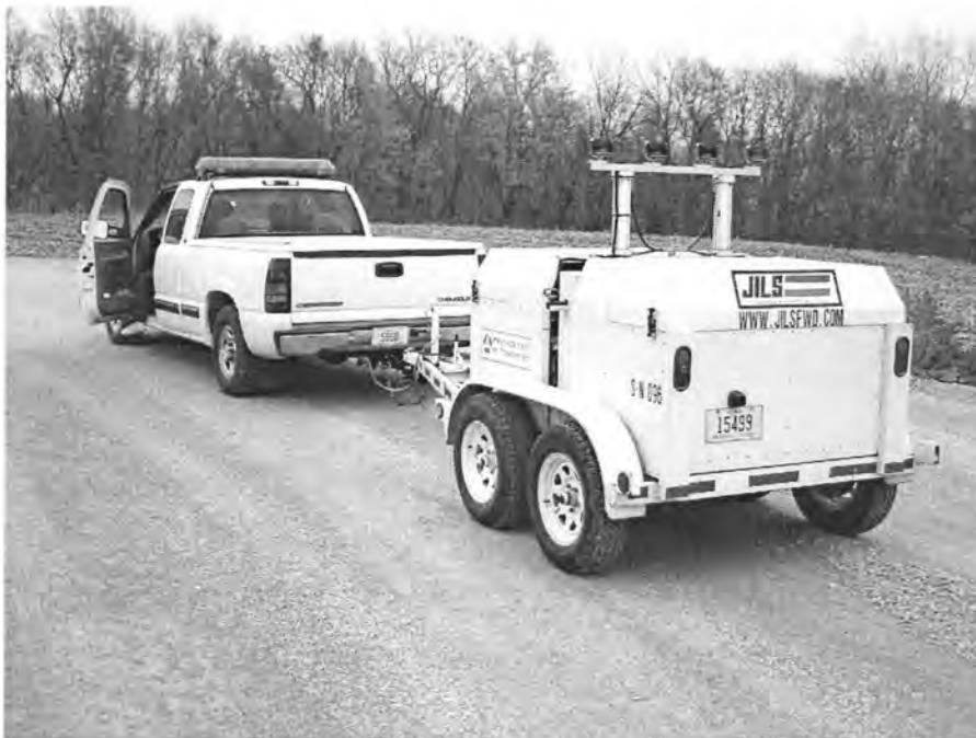
Figure 77. Falling Weight Deflectometer
